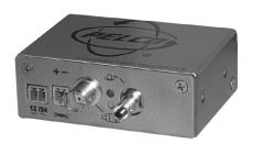
Specially designed for use in EH2515/EH3512/EH3515 Series camera enclosures and in DF5/DF8 Series fixed mount domes, the **FT8301A** transmitter can also be used as a standalone module. As a standalone module, the unit can be placed on a desktop or can be mounted to a wall.
