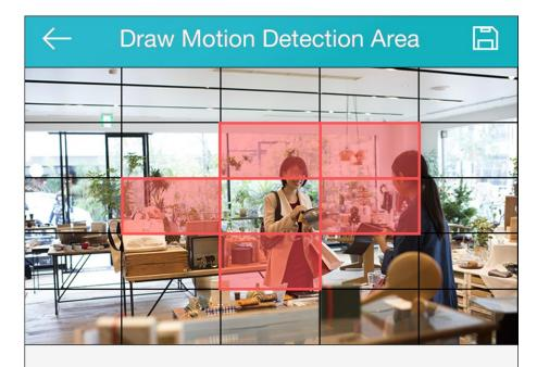
In the selected area, alarm and video recording will occur when the object is detected to move. in the horizontal screen mode, the area selection is more convenient
