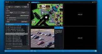
Event data received by the ARH system is displayed in the VX Ops Center. Critical event detail such as plate number, timestamp and snapshot overview are displayed side-by-side with live or recorded video from within the Ops Center. The integration of data makes it possible for real-time display of license plate information and real time alerts.
