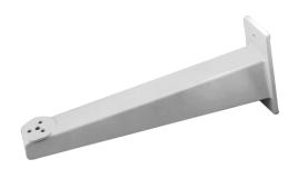
The **PM105** is a medium duty wall mount designed for mounting lightweight pan/tilts and is capable of handling loads up to 40 pounds (18.14 kg). The **PM105** can be used with the PT270P, PT270-24P, and PT280-24P pan/tilts.
