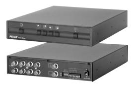
There are five alarm inputs, one for each of the four cameras, plus one for the quad input. When there is an alarm, that camera is switched to the call monitor's output for the duration of the alarm or until an operator acknowledges the alarm by pressing the front panel button associated with the alarmed camera. Multiple alarms will sequence at a two-second rate. An alarm output can trigger a VCR or an external alarm indicator, such as a light or buzzer.
