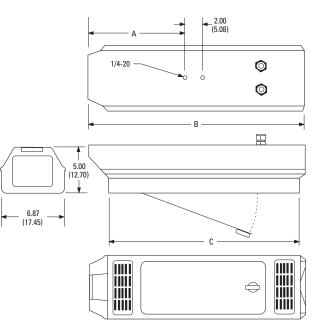
NOTE: EH4712DB SERIES DOES NOT HAVE VENTS IN BOTTOM OF ENCLOSURE.
