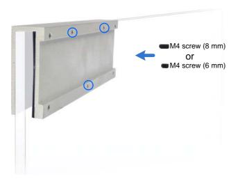
4. Place the Adjustable Plate on the Cover Plate. Adjust the position according to the GV-ML600 or GV-ML1200 electromagnetic lock's position on the opposite side of door frame.
