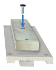
2. Attach the combination from Step 1 to the U bracket and secure it with M4 (11 mm) screws.
