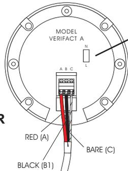
Microphone gain adjust: N is normal, L is low
