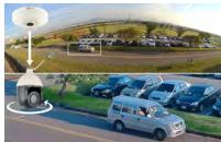
OZT technology combines three valuable features - Overview, Zoom and Tracking – to be able to automatically track any suspicious object over a wide area. The intelligent hemispheric camera with overview capability can be paired with a speed dome camera, and hence instructs the speed dome camera to zoom-in and track the object in a detailed manner.
