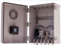
The AccelTex Solutions Heated & Cooled PoE enclosure allows an access point to be installed in an outdoor or other temperature-limiting environment. The heater, fan and AP are all powered by a single PoE cable run from the network switch. The enclosure ships ready for an AP and external antenna installation.
