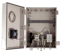
The AccelTex Solutions Heated & Cooled PoE enclosure allows an access point to be installed in an outdoor or other temperature-limiting environment. The heater, fan and AP are all powered by a single PoE cable run from the network switch. The enclosure ships ready for an AP and external antenna installation.
