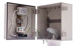
The AccelTex Solutions Heated PoE enclosure allows an access point to be installed in an outdoor or other temperature-limiting environment. The heater and AP are powered by a single PoE cable run from the network switch. The enclosure ships ready for an AP installation with our 2.4/5 GHz 4/6 dBi omni antenna integrated onto the bottom of the enclosure.
