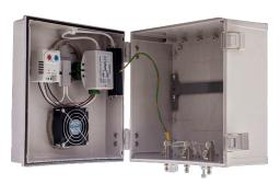
The AccelTex Solutions Heated & Cooled PoE enclosure allows an access point to be installed in an outdoor or other temperature-limiting environment. The heater, fan and AP are all powered by a single PoE cable run from the network switch. The enclosure ships ready for an AP and external antenna installation.
