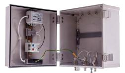
The AccelTex Solutions Heated PoE enclosure allows an access point to be installed in an outdoor or other temperature-limiting environment. The heater and AP are powered by a single PoE cable run from the network switch. The enclosure ships ready for an AP and external antenna installation.
