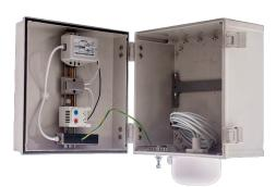
The AccelTex Solutions Heated PoE enclosure allows an access point to be installed in an outdoor or other temperature-limiting environment. The heater and AP are powered by a single PoE cable run from the network switch. The enclosure ships ready for an AP installation with our 2.4/5 GHz 4/6 dBi omni antenna integrated onto the bottom of the enclosure.
