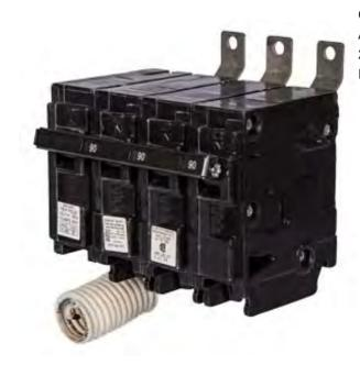
Siemens Low Voltage Molded Case Circuit Breakers Panelboard Mounting 240V Circuit Breakers - Type BL, 3-Pole, 240VAC are Circuit Protection Molded Case Circuit Breakers. Type: BL Application: Electrical Distribution Standard: UL 489 Voltage Rating: 240V Amperage Rating: 100A Trip Range: Thermal Magnetic Interrupt Rating: 10 AIC Number Of Poles: 3P
