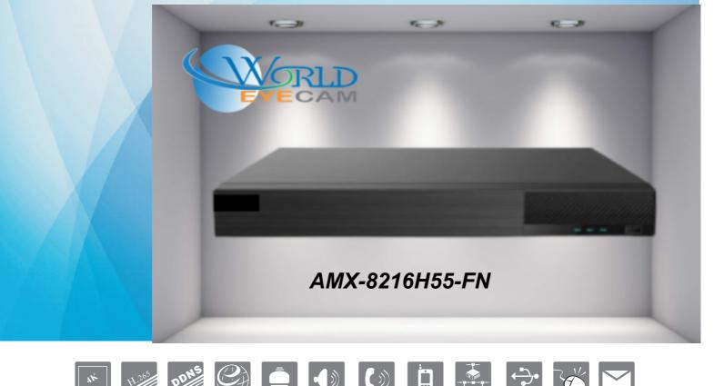
supports 8MP / 5MP / 4MP / 3MP / 1080P / 720P /WD1 analog and IP video input simultaneously. It adopts the standard H.265 high profile compression format and the advanced SOC technique to ensure real time recording in each channel and realize outstanding robustness of the system. ED8216H5-FN supports 16 CH analog video input, 8CH IP video input and 8CH audio input, simultaneous 16CH playback. The series of product can meet different security requirements of home,
