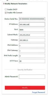
Figure 2-5 Modify the IP Address
