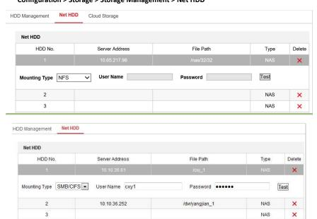
Figure 5-5 Select Net HDD Type
