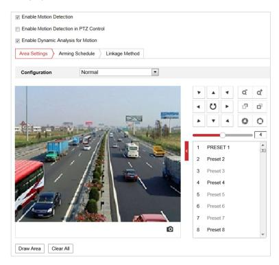
Figure 5-10 Motion Detection Settings-Normal
