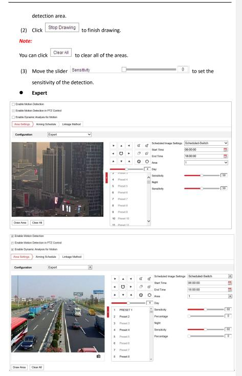
Figure 5-11 Motion Detection Settings-Expert
