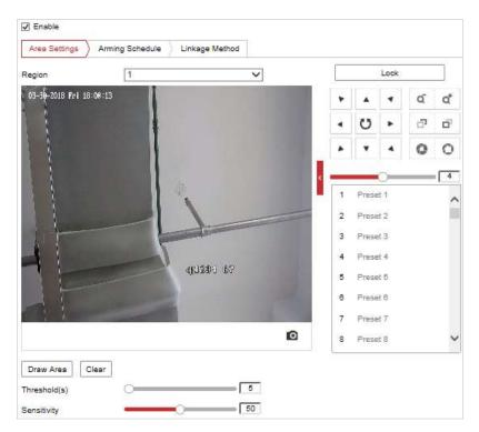
Figure 5-27 Configuring Region Exiting Detection
