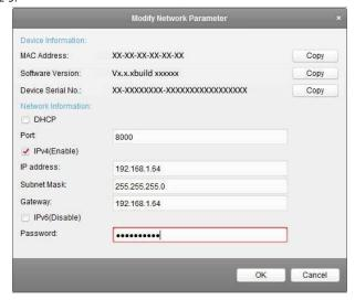
Figure 2-9 Modifying the Network Parameters
