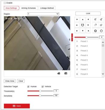
Figure 5-23 Configuring Intrusion Area
