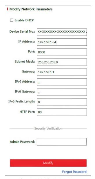
Figure 2-5 Modify the IP Address
