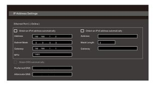
④ Go to Start → Settings → Camera → Add Camera. The NVR will automatically refresh the cameras searched. The IPC which supports the Onvif protocol may be added manually. If the IPC searched is not in the same local network as the NVR, you should select the device and click ■ to modify the IP address.
