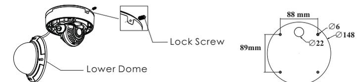
③ Route and connect these cables. Then secure the mounting base to the ceiling or wall with screws.
