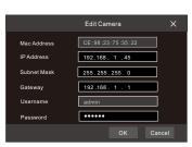
⑤ Checkmark the device you want to add and then click "Add" button. The DVR will automatically refresh the cameras and return to "Edit Camera" interface. "Online" status means connecting the device successfully and you will see the live image. You may select the added device and click ■ button to modify channel, IP address, ect.
