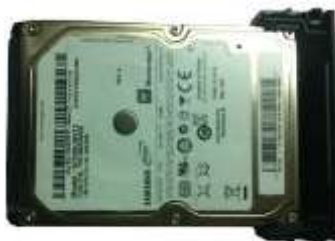
② Make sure the HDD metal surface is facing up and then put the HDD into the bracket horizontally. After the HDD is in the proper position, the columns on the two sides can lock the screw holes of the HDD to secure it.
