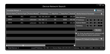
3 Modify the IP address. The default IP address of this camera is 192.168.226.201. Click the information of the camera listed in the above table to show the network information on the right hand. Modify the IP address and gateway of the camera and make sure its network address is in the same local network segment as the computer's. Please modify the IP address of your device according to the practical situation.
