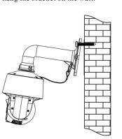
2. Secure the PTZ camera to the bracket with screws.
