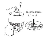
2. Insert a micro SD card as indicated above and then install the cover back.
