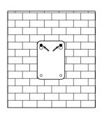
5. Connect the cables and then hang the bracket on the wall.
