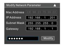
For example, the IP address of your computer is 192.168.1.4. So the IP address of the camera shall be changed to 192.168.1.X. After modification, please enter the password of the administrator and click "Modify" button to modify the setting.
