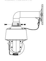
4. Insert two screws to the holes as indicated by the arrows (left) and leave 12mm clearance.
