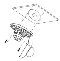
⑤ Three-axis adjustment. Before adjustment, preview the image of the camera on a monitor and then adjust the camera according to the figure below to get an optimum angle.
