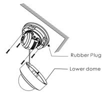
⑥ Three-axis adjustment. Before adjustment, view the image of the camera on a monitor and then adjust the camera according to the figure below to get an optimum angle.
