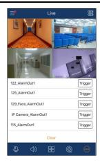
Select the desired alarm output and then click "Trigger" button to trigger alarm out manually. Click "Clear" to clear alarm output.
