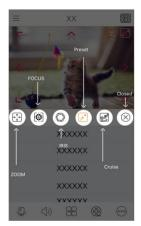
Please control the PTZ by sliding the image in direction of the arrow marked on the image. The PTZ will automatically focus on the little red circle by clicking the image. Then the 3D function can be enabled (the added device must be support 3D function, or this function is ineffective).
