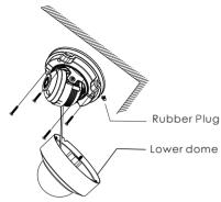
⑥ Three-axis adjustment. Before adjustment, view the image of the camera on a monitor and then adjust the camera according to the figure below to get an optimum angle.
