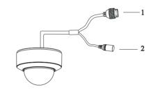
1 Ethernet connector 2 Power connector
