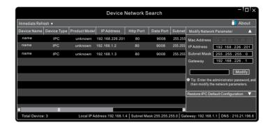
③ Modify the IP address. The default IP address of this camera is 192.168.226.201. Click the information of the camera listed in the above table to show the network information on the right hand. Modify the IP address and gateway of the camera and make sure its network address is in the same local network segment as the computer's. Please modify the IP address of your device according to the practical situation.
