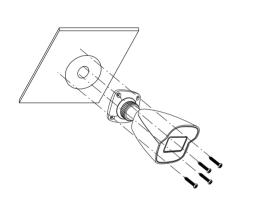
⑤ Bracket adjustment. Before adjustment, preview the image of the camera on a monitor and then loosen the fixed ring to adjust the view angle of the camera.
