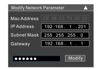
For example, the IP address of your computer is 192.168.1.4. So the IP address of the camera shall be changed to 192.168.1.X and the gateway shall be changed to 192.168.1.1. After modification, please enter the password of the administrator and click "Modify" button to modify the settings.
