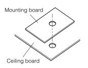
Attach the Ceiling Mount Ring (provided) to the Mounting board Screws are not provided. Align it with the position the camera will be installed.
