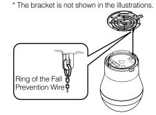
Attach the camera to the Camera Mounting Base, turn the camera clockwise, and tighten the Mounting Screw (M3, provided).
