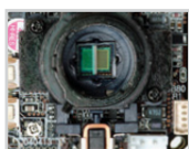
Mechanical IR Cutoff Filter
