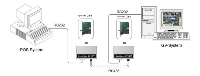
**Note:** For this connection, the maximum distance of RS232 is 10 meters (32 ft) while that of RS485 is 1200 meters (4000 ft).
