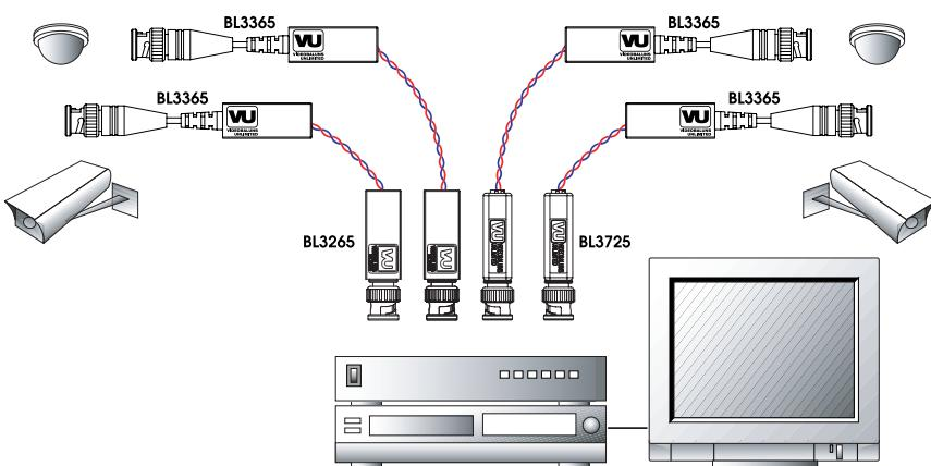
The EZ-VU video balun is designed to work in pairs. Models BL3365, BL3265, and BL3725 are functionally identical and are interchangeable.
