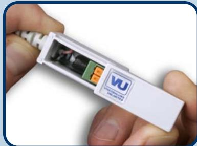
Slide off cover, Raise orange IDC Connectors and Insert wires.
