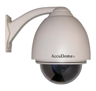
The aluminum cast structure, IP 66 weatherproof rated housing includes a built-in heater/blower assembly facilitating harsh winter environments. The WACD-1500-LG27's modular design guarantees efficient installation and service.
