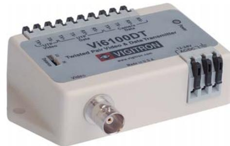
The Vigitron Vi6100DT is an advanced active device that transmits color or black and white video and data over separate point-to-point unshielded twisted pair wires at distances up to 6,000 feet (1,830 m). The Vi6100DT uses Category 2-7 twisted pair wires, is easy to install and cost effective. It is designed to be paired with Vigitron Vi6100DR active video and data receiver.
