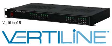
Altronix Vertiline16 CCTV Rack Mount Power Supply provides 16 fuse protected power outputs in a space saving 1U EIA 19" rack mount chassis which may be rack, wall or shelf mounted. This unit features individually selectable 24VAC and/or 28VAC power outputs with surge suppression. Vertiline CCTV Rack Mount Power Supplies are also available in eight (8) and twenty-four (24) output models with various power ratings.
