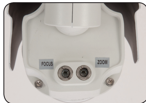
Gasket sealed externally adjustable Focus & Zoom with clutch to eliminate over-tightening.
