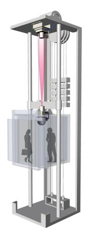
The VITEK VT-LTR13V-KIT is a laser optical video transmission system which was specifically designed for elevator CCTV surveillance applications. Because it transmits DVD quality video using a optical laser, cabling complexity, installation costs, and maintenance issues are drastically reduced. With a much longer life span than traditional 'moving coaxial cable' video transmission systems, the elevators operation, security, and safety is also increased.
