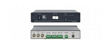
The VS-24xI is a high-performance switcher for composite and balanced stereo audio signals. When configured as a stand-by switcher, it switches to input 2 when the signal on input 1 is interrupted.
