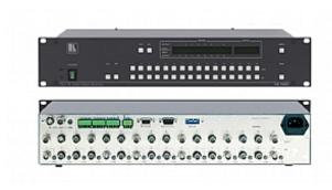
The VS-162V is a high-performance matrix switcher for composite video signals. It can also be configured as an 8x8 s-Video (Y/C) switcher, a 5x5 component (YUV) switcher, or a 4x4 RGBS switcher.
