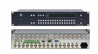
The VS-162AVRCA is a high-performance matrix switcher for composite video and unbalanced stereo signals. Switching during the vertical interval ensures glitch-free switching with genlocked sources.
