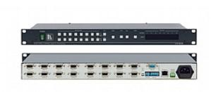
The VP-8x8 is a high-performance matrix switcher for computer graphics video signals, with resolutions up to and exceeding UXGA on 15-pin HD connectors. It can route any or all inputs to any or all outputs simultaneously.
