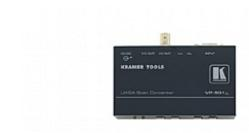
The VP-501xl is a scan converter for computer graphics video signals. It converts computer graphics video signals up to UXGA (1600x1200) to composite and s-Video (Y/C) signals simultaneously in either PAL or NTSC formats.
