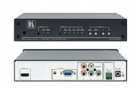
The VP-434 is a high-performance scaler for component video and computer graphics video with unbalanced stereo audio signals. It scales the selected video signal to a computer graphics or HDTV output resolution, embeds the audio and outputs an HDMI signal.
