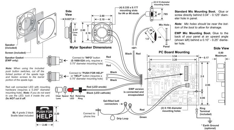
**Important:** If installing the **EWP** version outdoors, apply a non-corrosive silicone to back side of LED and push button switches after making all connections and testing. Completely encapsulate exposed switch connections (screw terminals/stripped wires) and bare wire connections.
