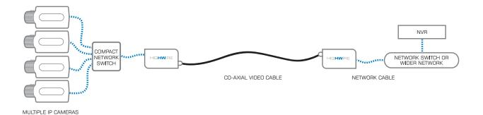
In this application, multiple IP cameras replace a single analog CCTV video camera. The IP cameras are connected to a small network switch. One port of the switch is linked to a HIGHWIRE device. Again, the HIGHWIRE link runs across the existing installed
