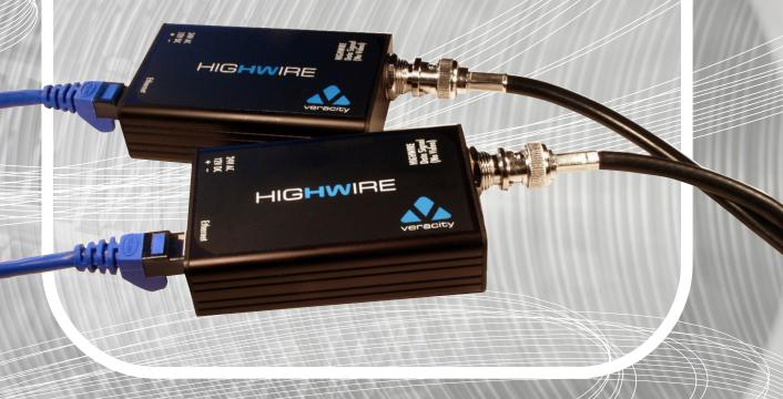
HIGHWIRE™ allows IP Network Cameras to communicate over existing co-axial video cables.
