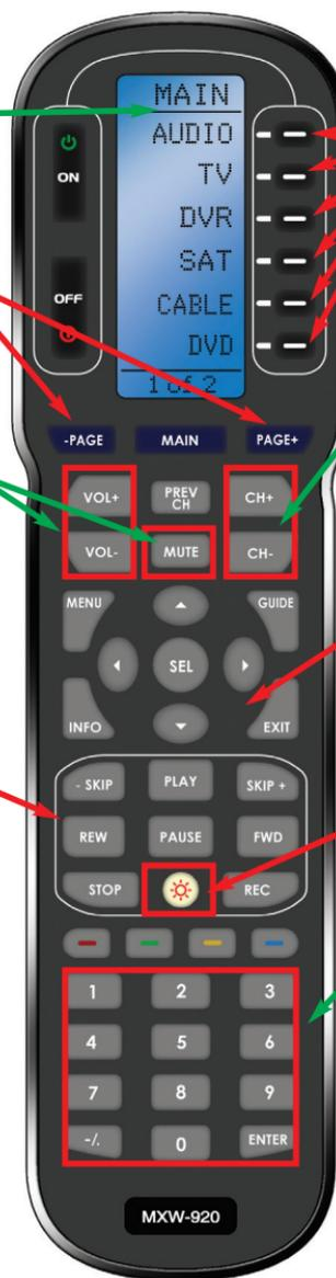
The **LCD button labels** describes the functions available for the current activity or device.
