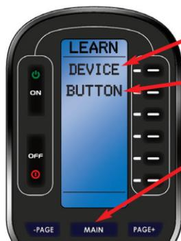
**Device** - Copy a command to a device button.
