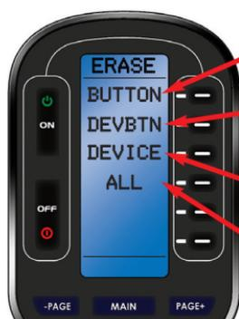
**Button** - Erases a specific command residing on a button within a device.
