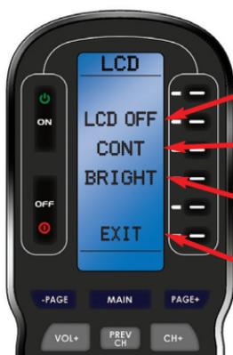
To activate the **LCD On/Off** setting, press this button. See below.
