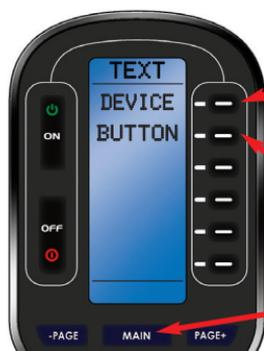
**Device** - Select a device to rename by pressing an adjacent button. Use the arrow and number buttons to add letters.
