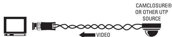
TW4001P AS RECEIVER CONNECTED TO OTHER UTP SOURCES
