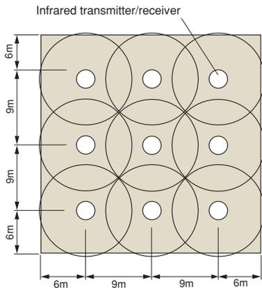
\*Choose the appropriate Transmitter/Receiver Unit according to the ceiling height.
