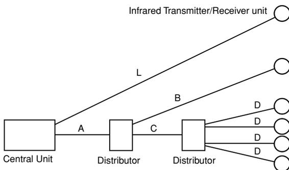
If two or more Infrared Transmitter/Receiver units with different connection cable lengths receive infrared signals from the Chairman and Delegate units, the signal reception level may decrease to cause malfunction.
