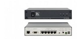
The TP-305A is a high-performance twisted pair receiver for computer graphics video, audio and RS-232 signals. The unit takes one twisted pair input and provides five twisted pair, a computer graphics video, stereo audio and S/PDIF audio outputs and an RS-232 output for local monitoring.
